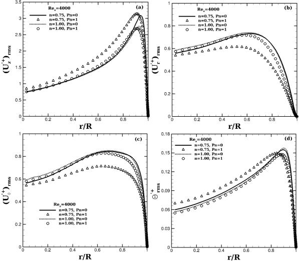
Figure 3. Root mean square of the fluctuating velocities and temperature,  $Pr_s = 1$ .
