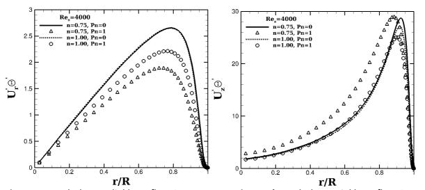
**Figure 4a.** Turbulent radial heat flux,  $Pr_s = 1$
