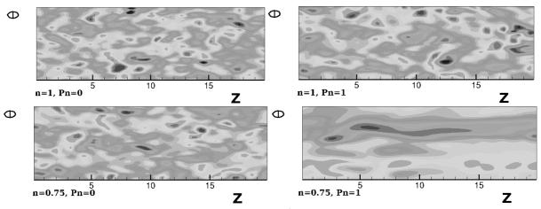
**Figure 5.** Resolved axial velocity fluctuations at  $Y^+ \approx 15$
