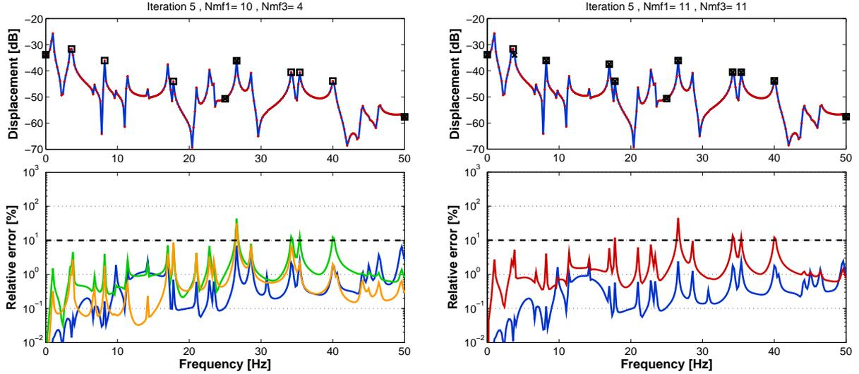
Figure 9: (top) FRF at the last iteration of the greedy algorithm, using the error indicator  $\tilde{\epsilon}_F$  (left) and the indicators  $\epsilon^1$  and  $\epsilon^3$  (right): — FE solution; ··· interpolated solution; □ master frequencies for substructure 1; × master frequencies for substructure 3. (bottom) relative errors: —  $\hat{\epsilon}_q(\omega)$ ; —  $\tilde{\epsilon}_F(\omega)$ ; —  $\tilde{\epsilon}^1(\omega)$ ; —  $\tilde{\epsilon}^3(\omega)$ ; - - - error threshold.
