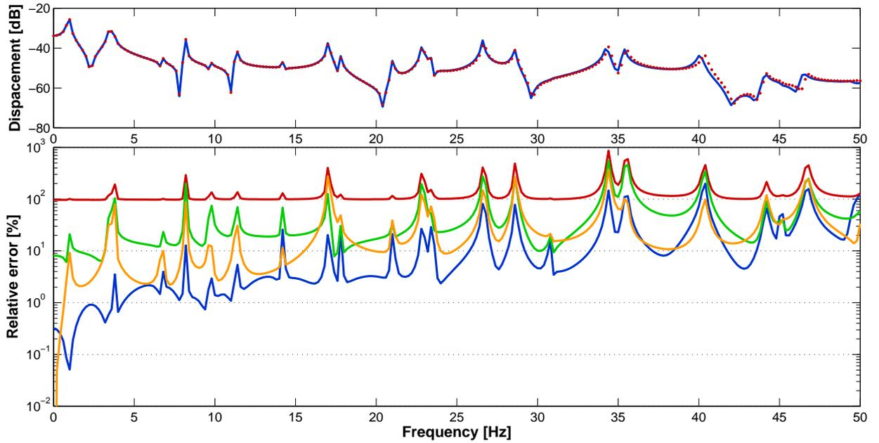
Figure 3: (top) FRF of the structure: — FE solution; ··· CB solution. (bottom) relative errors: —  $\tilde{\epsilon}_q(\omega)$ ; ···  $\tilde{\epsilon}_F(\omega)$ ; —  $\epsilon^1(\omega)$ ; —  $\epsilon^3(\omega)$ .
