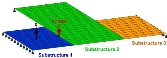
Figure 7: FE mesh of the three coupled plates structure with a 10N vertical point force acting on the interface between substructures 1 and 2, and a response measurement point in substructure 1.
