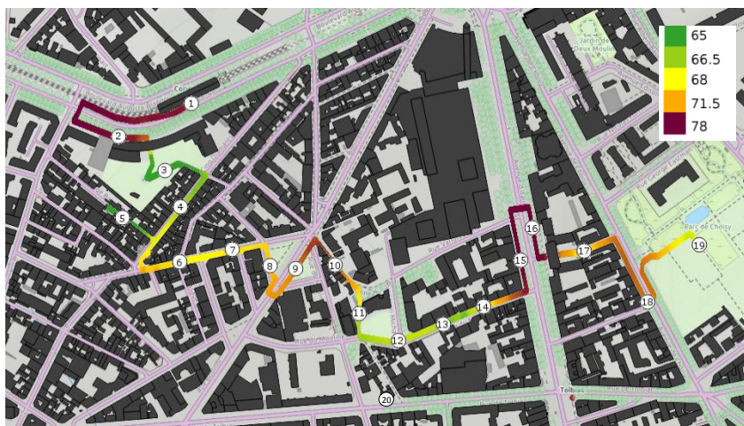
Figure 1: Noise Map of the studied path, interpolated from mobile measurements (LAeq - dB).
