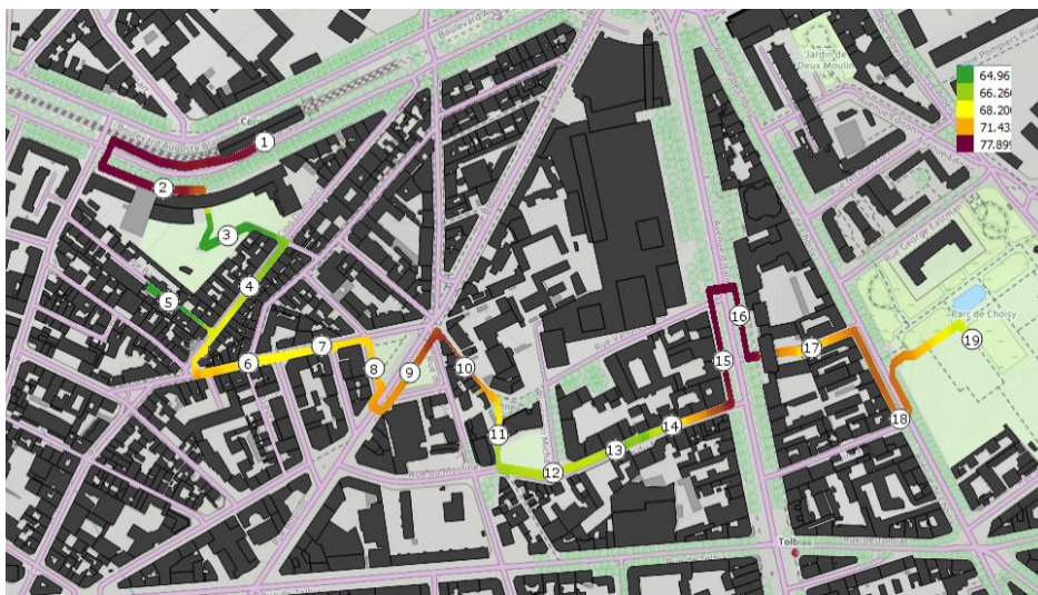
Figure 1 Noise Map of the studied path, interpolated from mobile measurements (Leq - dB)
