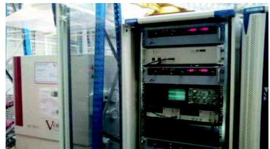
Fig. 2. Climatic chamber and power electronics as a test bench for the insulation materials.
