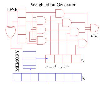
Fig. 1. Hardware implementation of the Conditional Distribution Element.
