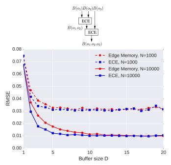
Fig. 2. The bitstream  $B(o_1.o_2.o_3)$  is computed, the odds of which are the product of the three input stream odds  $o_1$ ,  $o_2$  and  $o_3$ , which correspond to probability values uniformly drawn between 0 and 1. The RMSE is experimentally computed for buffer sizes ranging from 1 to 20, over 10000 runs. As usual with stochastic computing, the precision depends on the size N of the bitstream (here 1000 or 10000) and goes as  $\frac{1}{2/N}$ .
