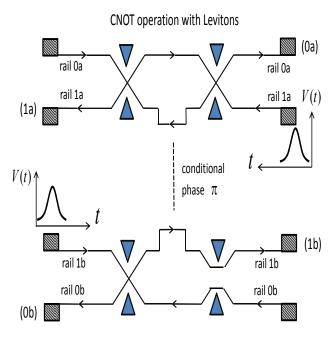
**Figure 9** Schematic representation of a CNOT quantum gate with Levitons. Two Levitons are injected in rail 1a and 1b. The output state is a maximally entangled state. The vertical dashed line schematically indicates the Coulomb interaction which could provide a conditional  $\pi$  phase shift in the two particle (two-qubit) wavefunction.
