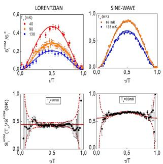
**Figure 6** Temperature dependence of the HOM shot noise for lorentzian (left) and sinewave (right) pulses. By plotting the ratio of the HOM noise to the theoretical zero temperature HOM noise versus the HOM delay  $\tau$ , one observes that, contrary to the sinewave pulses, for levitons the HOM noise shape versus  $\tau$  is not affected by thermal excitations. Figures adapted from [41]
