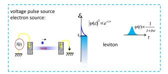
**Figure 2** Top figure: the mesoscopic capacitor source (energy-resolved source). Its energy distribution is lorentzian and the time wavepacket envelope is semi-exponential. Bottom Figure: the voltage pulse leviton source. Its energy distribution is semi exponential and the time wavepacket is lorentzian. The two sources are suitable for electron quantum optics. They show a duality when interchanging time and energy
