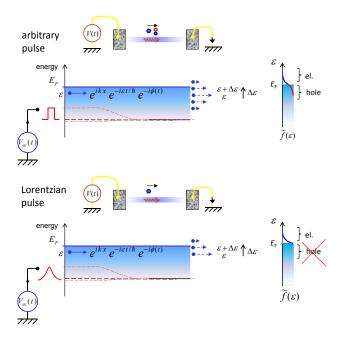
**Figure 3** Top figure: effect of an arbitrary pulse on the Fermi sea. Electrons are scattered to different energies above and below their initial energy. Electron hole excitations are created, as schematically represented in the energy distribution  $\widetilde{f}(\varepsilon)$ . Bottom figure: applying a Lorentzian shape voltage pulse generates a minimal excitation state called Leviton , no hole excitation is created.
