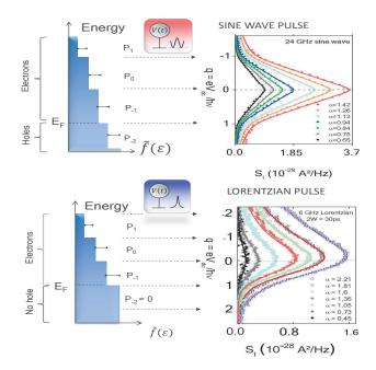
**Figure 4** Top figure: shot noise spectroscopy of a sine wave pulse. Since an equal number of electron and hole excitations is created the noise spectroscopy is symmetric with respect to  $V_R=0$ . The schematic zero temperature energy distribution  $\widetilde{f}(\varepsilon)$  is shown on the left. Bottom figure: shot noise spectroscopy of a lorentzian pulse. The number of holes is minimized to zero and the shot noise spectroscopy is asymmetric. The figures are adapted from [23]
