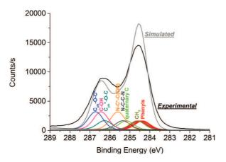
FIG. 3. C1s spectra decomposed using the  $\Delta BE(\Delta SCF)$  results along with the actual stoichiometry.
