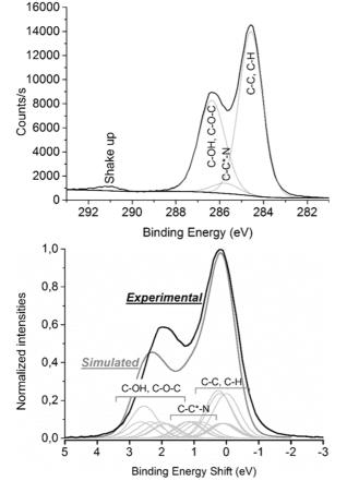
FIG. 2. (a) Experimental C1s spectrum decomposed empirically. (b) Comparison of the experimental and simulated C1s spectra obtained from the sum of the calculated contributions of each orbitals.
