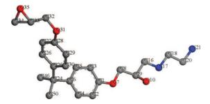
FIG. 1. Model dimer made of 1 diglycidylether of bisphenol A (DGEBA) and 1 ethylene diamine (EDA) molecules, through the reaction of one  $NH_2$  proton of EDA that opens one epoxy ring of DGEBA. H atoms are not shown for clarity.
