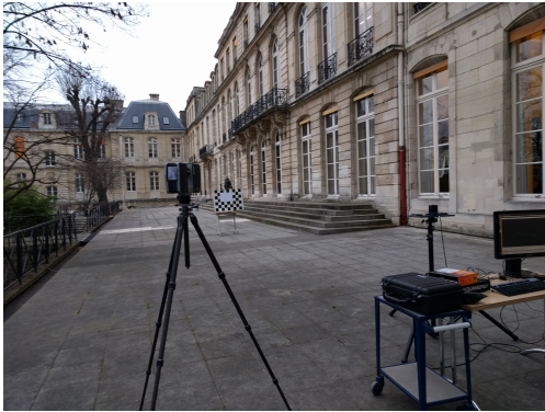
Figure 7: Experience on the evaluation of the accuracy of the distance measurement (outdoor)
