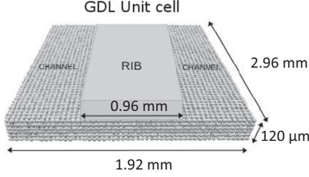
**Fig. 6.** Sketch of cubic network used to represent the GDL. The lattice spacing  $a_{ij}$  (distance between two neighbor pore) is  $80 \mu\text{m}$  in the plane directions. The GDL is represented by a  $25 \times 38 \times 4$  cubic network.
