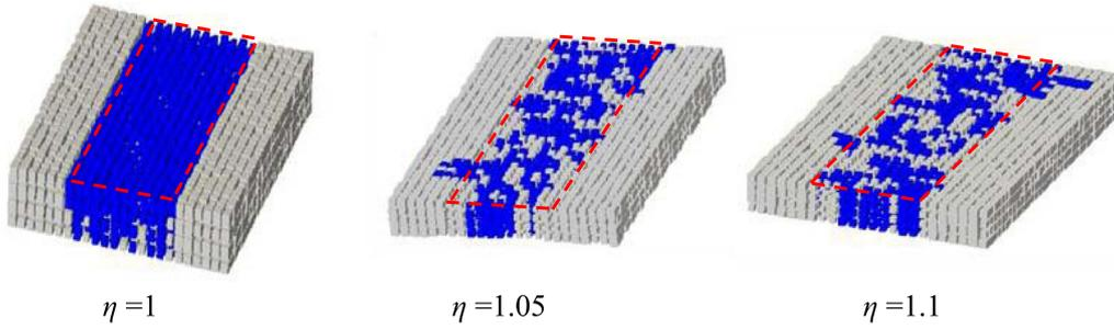
**Fig. 16.** Impact of nucleation parameter. Images of the distribution of the liquid water (in blue) in the GDL for the reference case ( $\eta = 1$ ) and for  $\eta = 1.05$  and  $\eta = 1.1$ ;  $i = 1.5 \text{ A/cm}^2$ ,  $RH_{ch} = 90\%$ . The red dashed lines materialize the position of the rib. (For interpretation of the references to colour in this figure legend, the reader is referred to the web version of this article.)
