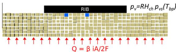
**Fig. 7.** Sketch of nucleation step. Sketch of two nucleation pores (in blue) under the rib. (For interpretation of the references to colour in this figure legend, the reader is referred to the web version of this article.)
