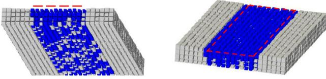
**Fig. 11.** Two images of the liquid water (in blue) distribution in the GDL for the reference case ( $i = 1.5 \text{ A/cm}^2$ ,  $RH_{ch} = 90\%$ ). The red dashed lines materialize the position of the rib. (For interpretation of the references to colour in this figure legend, the reader is referred to the web version of this article.)
