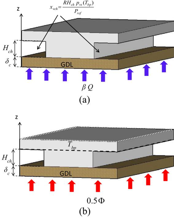
**Fig. 4.** Schematic drawing of studied problem. (a) water transfer problem: a fraction of the water produced in the catalyst layer is directed toward the cathode GDL; given relative humidity and total gas pressure are imposed in the channels, (b) heat transfer problem: a heat flux is applied at the GDL inlet whereas the temperature  $T_{bp}$  is imposed all over the surface in the  $x$ - $y$  plane at the position  $z = \delta_c + H_{ch}$ .
