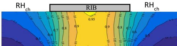
**Fig. 9.** Example of local relative humidity distribution in a  $x$ - $z$  plane cross section of the network in the absence of condensation. This field was computed for  $i = 1$  A/cm<sup>2</sup>,  $T_{bp} = 80$  °C and  $RH_{ch} = 50\%$ . Note that the through-plane scale is dilated for clarity. The GDL appears much thicker than it is actually.
