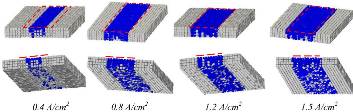
Fig. 14. Impact of current density. 3D images of phase distributions (liquid water in blue). The red dashed lines materialize the position of the rib.  $RH_{ch} = 90\%$ . (For interpretation of the references to colour in this figure legend, the reader is referred to the web version of this article.)
