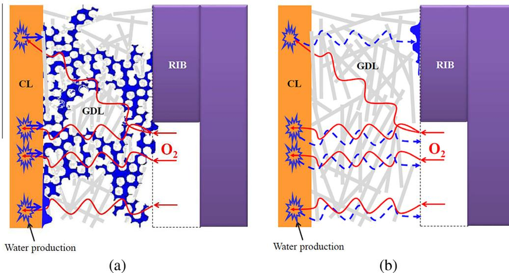
**Fig. 1.** Schematic of the two main situations regarding the phase, liquid or vapour, of the water entering the GDL from the catalyst layer (CL); (a) assumption #1: water enters the GDL in liquid form (in blue), (b) assumption # 2: water enters the GDL in vapour form (blue dashed lines). (For interpretation of the references to colour in this figure legend, the reader is referred to the web version of this article.)
