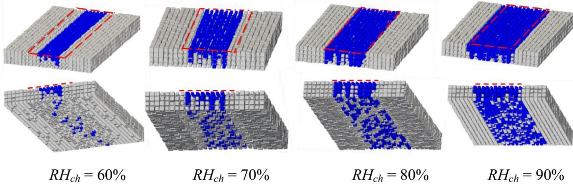
**Fig. 12.** Impact of channel relative humidity. 3D images of phase distributions. (liquid water in blue). The red dashed lines materialize the position of the rib.  $i = 1.5 \text{ A/cm}^2$ . (For interpretation of the references to colour in this figure legend, the reader is referred to the web version of this article.)
