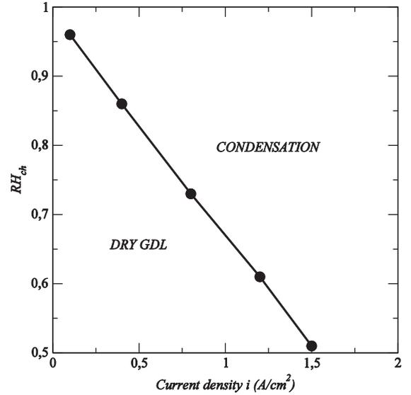
**Fig. 10.** Condensation diagram obtained for the polarization curve depicted in Fig. 2 and  $T_{bp} = 80$  °C and  $P_{ref} = 1.5$  bar. The water produced in the catalyst layer can be entirely transferred in vapour phase through a fully dry GDL for the operating points located below the curve. Liquid water formation occurs in the GDL for the operating points located above the curve.
