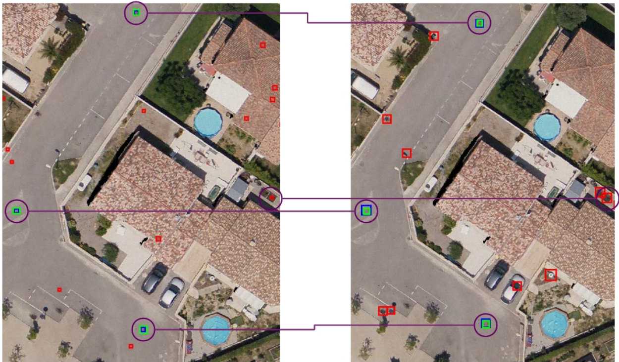
Figure 5: The two figures represent the results obtained with the circular filter on the left and the machine learning method on the right. The red rectangles are the true negatives, the blue rectangles are the true positives and the green rectangles are the ground truth. The lines connect the two common results between two approaches. The testing image is at 4 cm resolution.
