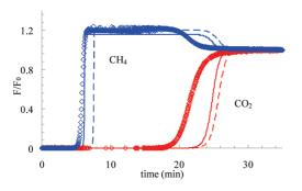
Figure 5. Breakthrough curves of the CO<sub>2</sub>-CH<sub>4</sub> equimolar mixture at 303 K and 0.1 MPa on the Cu-BTC: experimental data (diamonds), simulated data based on pure component isotherms (dashed line), and simulated data based on coadsorption isotherms (full line).
