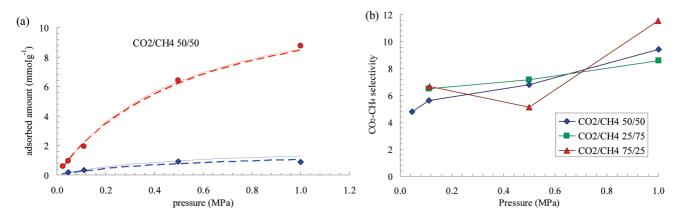
Figure 4. (a) Co-adsorption isotherm of the equimolar mixture of CO<sub>2</sub> (circles) and CH<sub>4</sub> (diamonds) at 303 K. Full lines represent the Langmuir model based on single-component isotherms; dashed thick lines, ideal adsorbed solution theory (IAST); dashed thin lines, the Langmuir model based on binary breakthrough experiments. (b) CO<sub>2</sub>-CH<sub>4</sub> selectivity as a function of pressure for the three gas mixtures.
