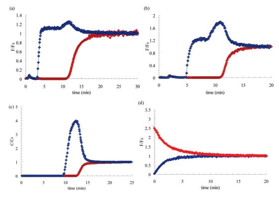
Figure 3. Breakthrough curve of CO<sub>2</sub> (red) and CH<sub>4</sub> (blue) at 0.5 MPa and 303 K for the 25-75 CO<sub>2</sub>-CH<sub>4</sub> mixture (a), 50-50 mixture (b), and the 75-25 mixture (c) and the 50-50 mixture on a column presaturated with CO<sub>2</sub> (d).
