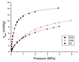
Figure 2. Absolute adsorbed amounts of pure CO<sub>2</sub> (full squares), CH<sub>4</sub> (open squares), and CO (triangles) at 303 K and the corresponding Langmuir (for CO<sub>2</sub> and CH<sub>4</sub>) and Langmuir-Freundlich fits (for CO).
