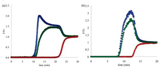
Figure 6. Breakthrough curve of CO<sub>2</sub> (red), CH<sub>4</sub> (blue), and CO (green) at 0.1 (a) and 1.0 MPa (b) at 303 K for the 70-15-15 CO<sub>2</sub>-CH<sub>4</sub>-CO mixture.
