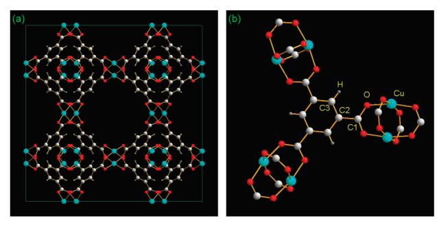
Figure 1. (a) Unit cell crystal structure of the Cu-BTC along the [100] direction. (b) Cluster of the Cu-BTC. (Cu, green; O, red; C, white; H, gray).
