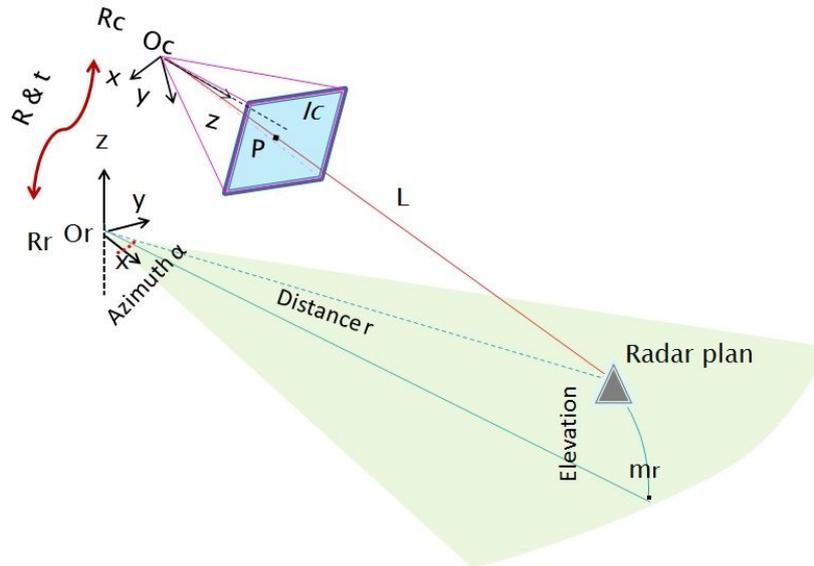
**Figure 1.** Sensors system geometry:  $R_c$  and  $R_r$  are the camera and radar frames, respectively. Polar coordinates  $m_r(\alpha, r)$  of the target are provided by the radar data, but not the elevation angle. The light ray  $L$  and the projected point  $p$  in the image  $I_c$  are shown together with the horizontal radar plane.
