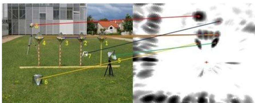
**Figure 19.** An image and a panoramic of targets. The targets are numbered from 1 to 8: one Luneburg lens and seven trihedral corners. The yellow crosses indicate the centers of the targets. The variations of amplitude of the reflected signal are introduced by the nature and orientation of each target. Manually-extracted matches between the image and the PPI are shown.
