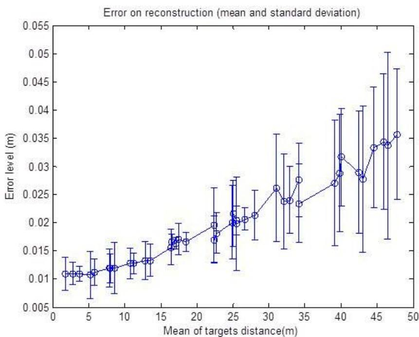
**Figure 16.** Reconstruction error with respect to the mean depth of the targets with a noise level corresponding to  $\pm 2 p$ ,  $\pm 2^\circ$  for  $\alpha$  and  $\pm 2$  cm for  $r$ . The error is in meters. The mean and standard deviation of the RMSE, over 50 reconstructed points, are shown.
