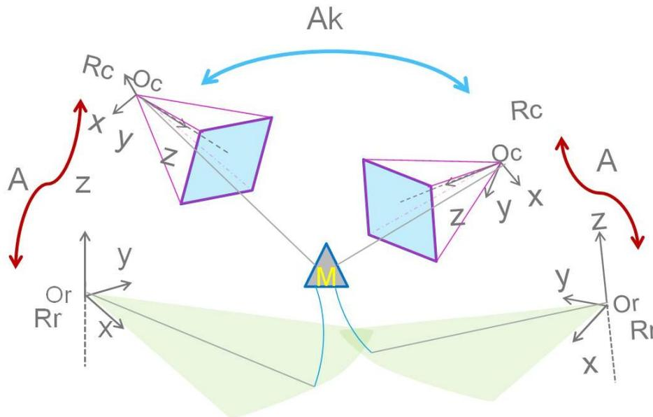
**Figure 6.** The displacement of the system around a fixed scene gives more geometric equations. An illustration of this process is shown. The matrix  $A_k$  represent the transformation between one position and another.
