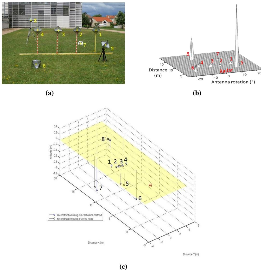
**Figure 20.** Reconstruction results using the inter-distance constraint for calibration. (a) Camera image of the eight canonical targets: one Luneburg lens and seven trihedral corners. The yellow crosses indicate the center of the targets; (b) Radar image with eight canonical targets; (c) The reconstruction results of both of our reconstruction methods (circular points) and the stereo head method as the ground truth (squared points). The radar position is indicated by the letter R.
