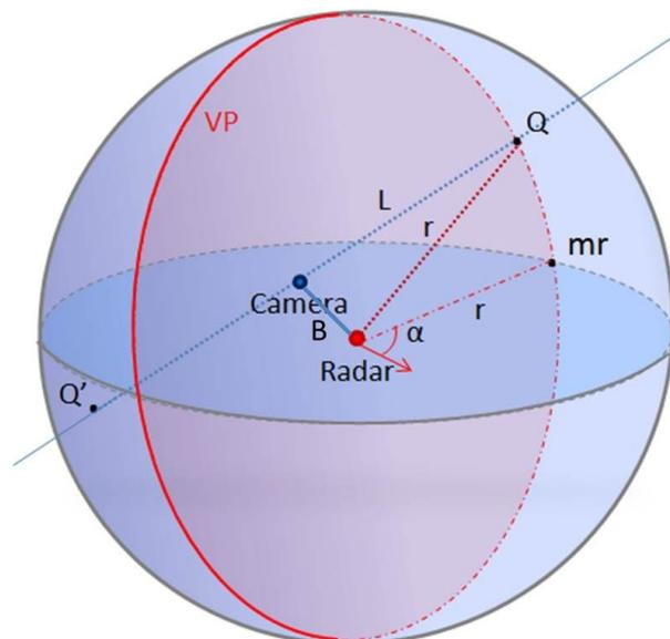
**Figure 4.** The 3D reconstructed point  $Q$  is the intersection of light ray  $L$  and the sphere  $C$  at  $\alpha$ .  $m_r$  is the projected 2D point on the horizontal radar plane, and  $VP$  is the vertical plane of the target at  $\alpha$ .
