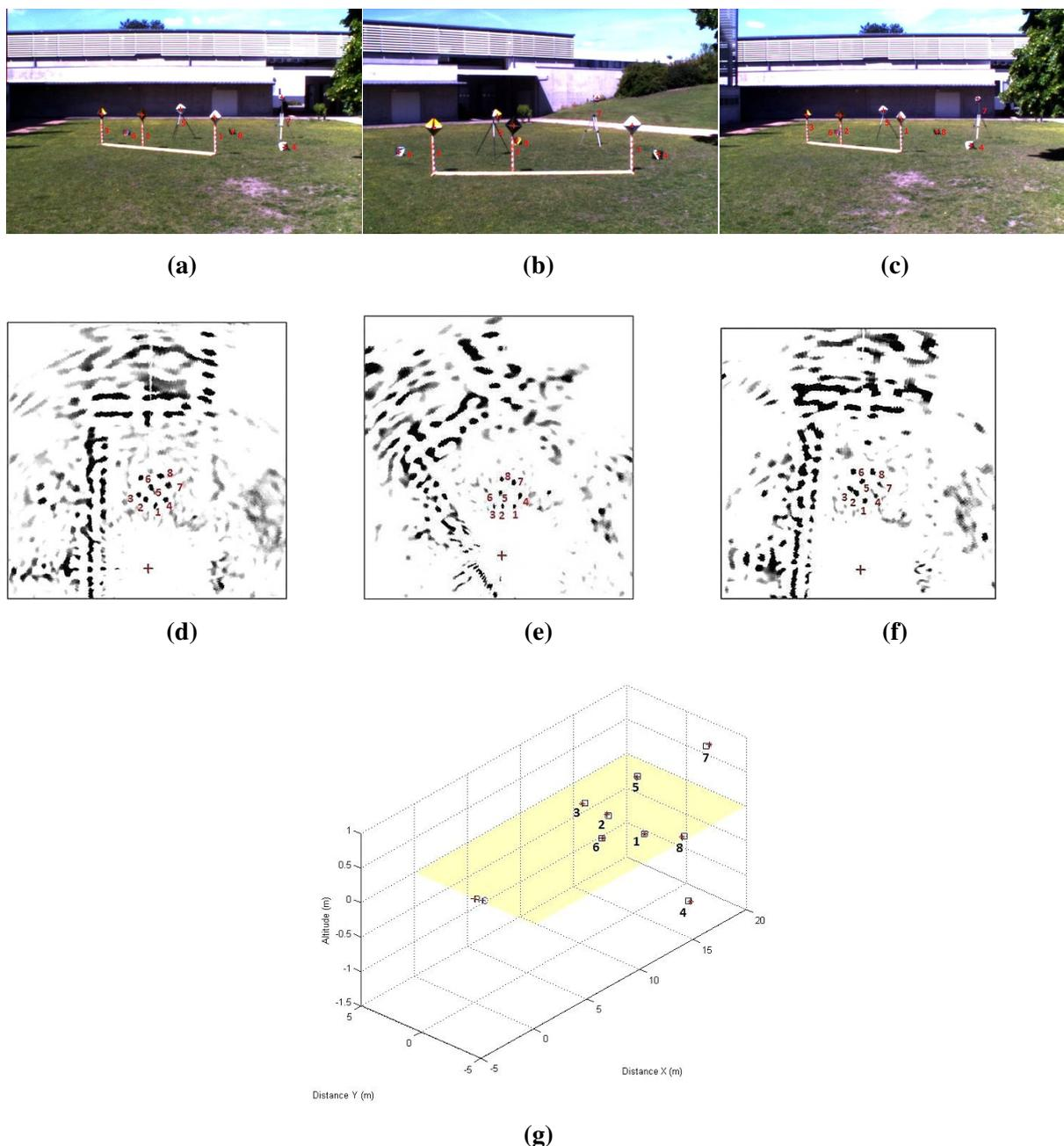
**Figure 21.** Top line: Camera images of the eight canonical targets. middle line: Radar images with eight canonical targets. The reconstruction results from both our reconstruction methods (circular points) and the stereo head method as the ground truth (squared points). The radar position is indicated by the letter R. (a) First position; (b) Second position; (c) Third position; (d) First position; (e) Second position; (f) Third position; (g) Reconstruction results.
