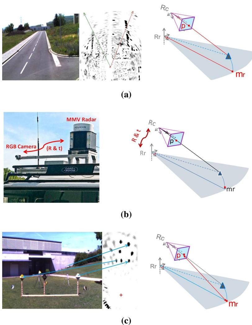
**Figure 3.** In order to achieve the 3D reconstruction, three preliminary steps must be carried out: simultaneous data acquisition by the sensors, the estimation of the transformation between the sensor frames and the extraction and matching of features from the camera image and the radar panoramic. (a) Data acquisition; (b) System calibration; (c) Features extraction and matching.
