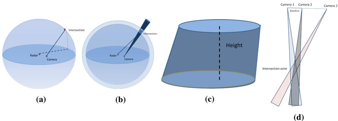
**Figure 13.** The intersection of the uncertainty regions of each sensor’s projection: (a) the ideal case of the geometric reconstruction; (b) introducing uncertainty regions of each sensor to the geometric model; (c) the error intersection region; (d) uncertainty intersection region in respect to the baseline for the stereo reconstruction method.
