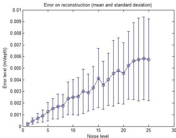
**Figure 9.** Reconstruction error with respect to the noise level. The error is in meters relative to the point depths  $r$ . The mean and standard deviation of the RMSE, over 50 reconstructed points, are shown.
