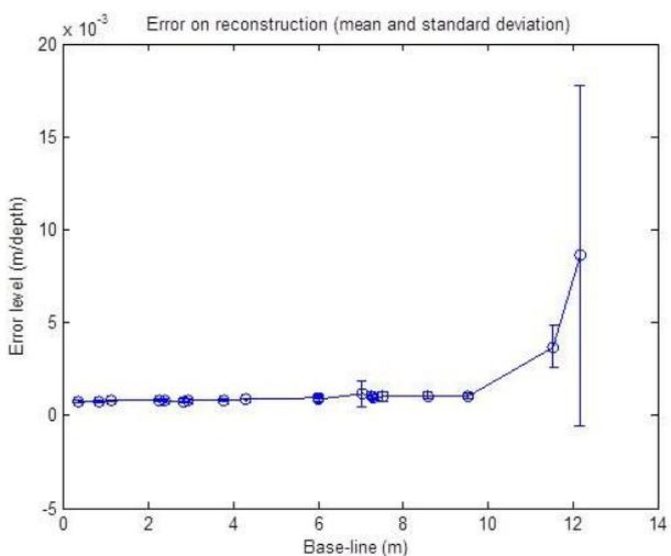
**Figure 10.** Reconstruction error with respect to the baseline with a noise level corresponding to  $\pm 2$  p,  $\pm 2^\circ$  for  $\alpha$  and  $\pm 2$  cm for  $r$ . The error is in meters relative to the point depths ( $r$ ). The mean and standard deviation over 50 reconstructed points are shown.
