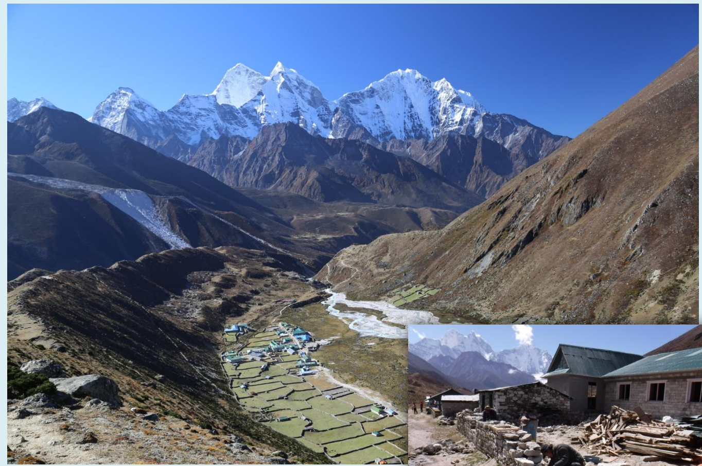
The high Sherpa village of Pheriche is located on a glacial ground moraine surrounded by high lateral moraines. Ground shaking of water-saturated glacial sediment resulted in significant damage (inset photo).
