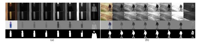
Figure 6: Visual results of the proposed method on each RGB and multispectral bands. From top to bottom: input image, *low-rank* component, *sparse* component, and the foreground mask. From left to right: RGB image, set of 7 visible, and 1 NIR spectrum are shown in each of columns respectively.
