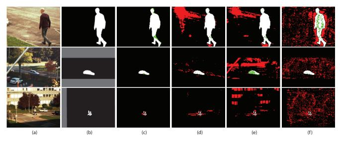
Figure 5: Visual comparison of background subtraction results over three scenes of the MSVS data set [1]. From left to right: (a) input image, (b) ground truth, (c) proposed approach, (d) BRTF [29], (e) HORPCA [7], and (f) CP-ALS [15]. The true positives (TP) pixels are in white, true negatives (TN) pixels in black, false positives (FP) pixels in red and false negatives (FN) pixels in green.
