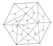
FIGURE 2. The triangular mesh  $\mathcal{T}$  (solid line) and its corresponding dual barycentric dual mesh  $\mathcal{M}$  (dashed line).
