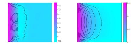
FIGURE 4. Test 3: 2nd mesh and anisotropic tensor  $\Lambda_{xx} = 1$  and  $\Lambda_{yy} = 100$ . Discrete solutions  $s_{\mathcal{M},\Delta t}(\cdot, t_f)$  and their iso-values. *Left:* Quasilinear scheme (71). *Right:* Nonlinear scheme (63).
