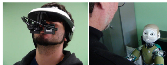
Figure 10. Immersive teleoperation of the GIPSA-Lab humanoid robot NINA. The pilot (left) communicates through the sensors (ear microphones and micro cameras embedded in the robot's eyes) and the actuators (neck, eyes, jaw, lips, etc.) of his robotic surrogate (right) with a remote interlocutor.
