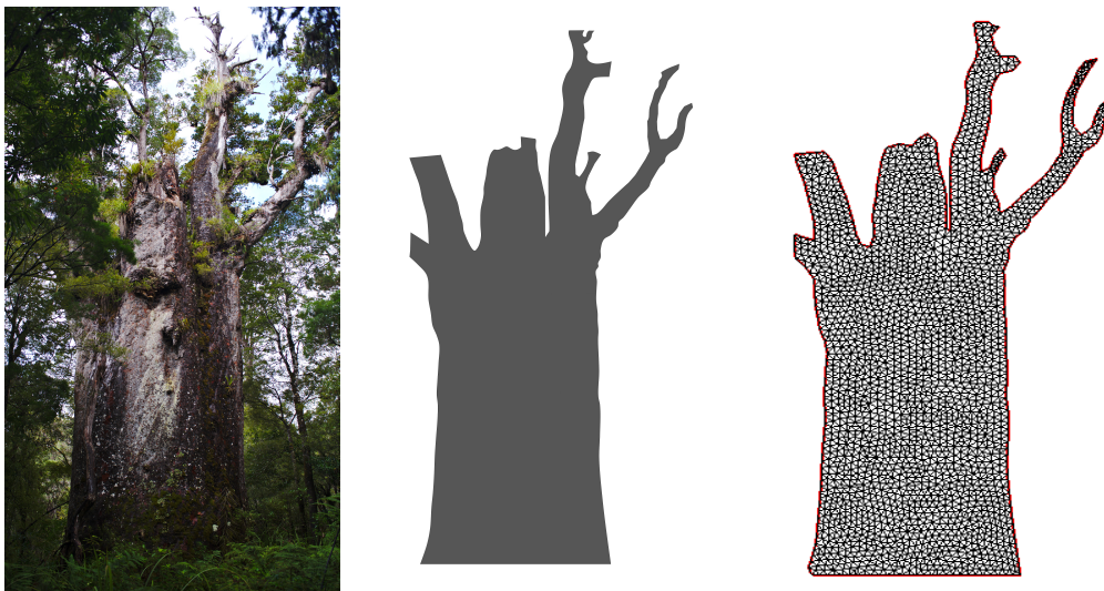
Figure 5: Mesh reconstruction of Te Matua Ngahere from a photograph (credit: D. Sellier).
