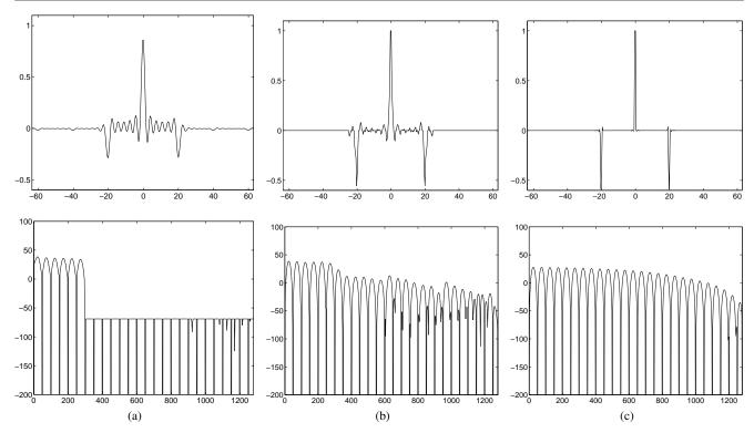
Fig. 3 State-of-the-art results: pulse x (top) and its Fourier transform  $\chi$  (bottom). (a) Minimizer of  $\|x\|_2^2 + d_{C_3}(x) + d_{C_4}(x)$  subject to  $x \in \left(\bigcap_{k \in \mathbb{D}_1} C_1^{(k)}\right) \cap C_2$ . (b) Minimizer of  $\|x\|_2^2 + \sum_{k \in \mathbb{D}_1} d_{C_1^k}^2(x)$  subject to  $x \in C_2 \cap C_3 \cap C_4$ . (c) Minimizer of  $\|x\|_2^2$  subject to  $x \in C_2 \cap C_3 \cap C_4$ .
