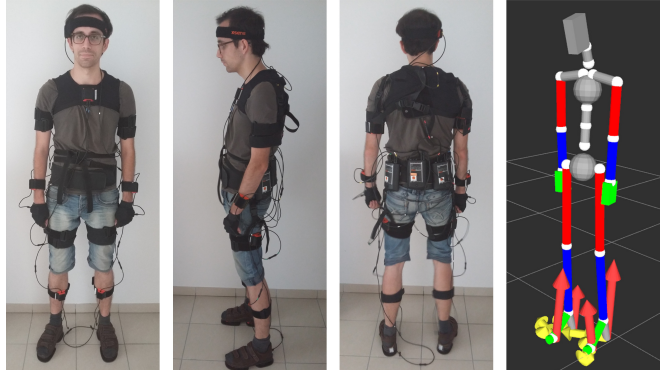
(a) Motion capture suit, contact force (red) and torque (yellow) visualization.
