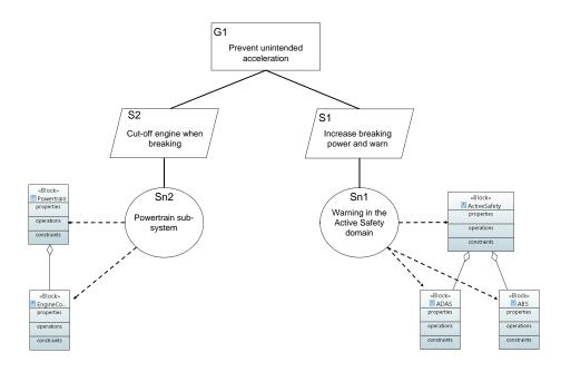
Fig. 6. Example of a safety view combining two notations.
