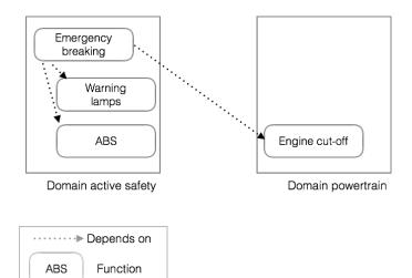
Fig. 2. Example of a functional architecture - or a functional view.
