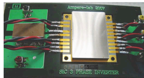
Figure 10: A JFET-based, 540 V, 15 A, 3-phase inverter in a single package with an external DC capacitor.
