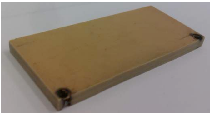
Fig. 6: Assembled passive substrate with embedded transformer
