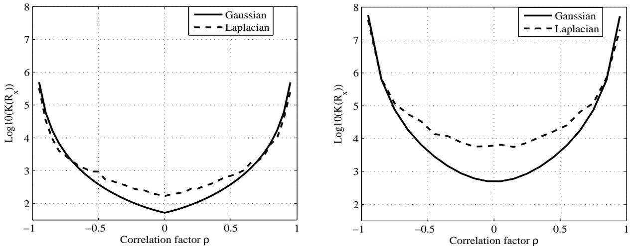
Fig. 2. Condition number of the estimated matrix  $\hat{\mathbf{R}}_{\mathbf{x}}$  (50.000 samples) according to the correlation factor  $\rho$ , for Volterra systems  $S_1$  (left,  $M = 2$  and  $N = 3$ ) and  $S_2$  (right,  $M = 2$  and  $N = 2$ ).
