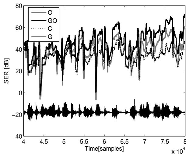
Fig. 14. NL system with memory ( $N = 3$ ,  $M = 50$ ), exact modeling case: Signal to Error Ratio for the classical and the proposed identification methods, for speech with and without Gaussianization ( $\mu = 0.1$ ,  $SNR = 40$  dB and  $\chi = -18$  dB).
