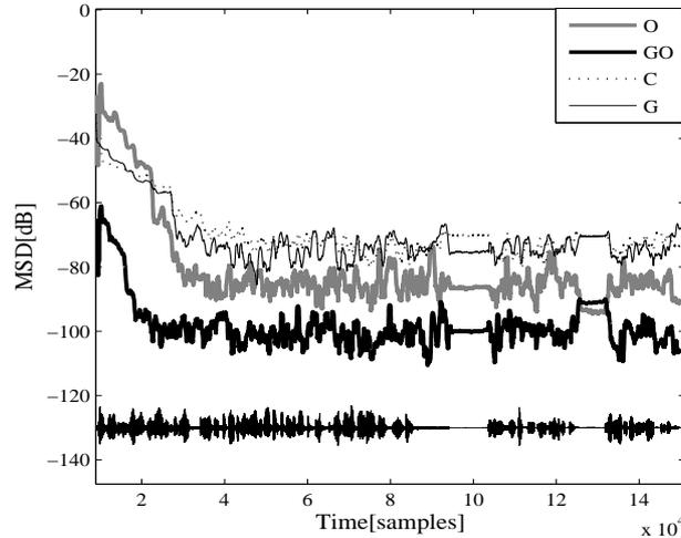
Fig. 11. For a system with memory, MSD time variation for classical identification and for the proposed method, for original speech and Gaussianized speech ( $\mu = 0.1$ ,  $N = 3$ ,  $M = 3$ ,  $SNR = 40$  dB and  $\chi = -18$  dB).
