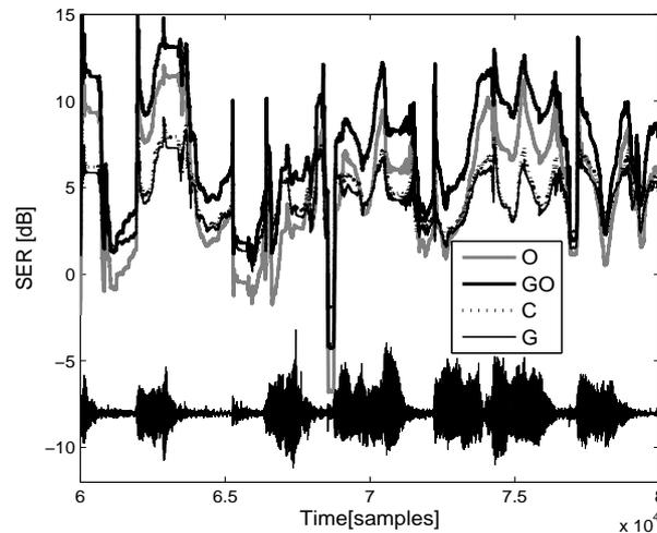
Fig. 15. NL system with memory ( $N=3$ ,  $M=50$ ), under-modeling case ( $N = 2$ ,  $M = 40$ ): Signal to Error Ratio for the classical and the proposed identification methods, for speech with and without Gaussianization ( $\mu = 0.1$ ,  $SNR = 40$  dB and  $\chi = -18$  dB.)
