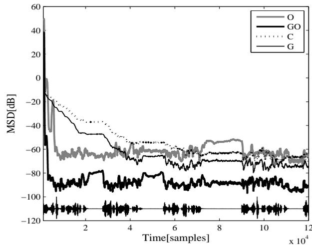
Fig. 9. For a polynomial system, MSD time variation for classical identification and for the proposed method, for original speech and Gaussianized speech. ( $N = 7$ ,  $\mu = \mu^o = 0.02$ ,  $SNR = 40$  dB and  $\chi = -18$  dB).
