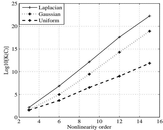
Fig. 1. For a polynomial system, condition number  $K(C_x)$  according to the nonlinearity order, for different generalized Gaussian processes.
