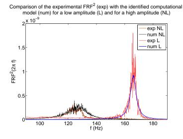
Figure 6: Comparison of the experimental  $FRF^2$  (exp) with the identified computational model (num) for a low amplitude (L) and for a high amplitude (NL).
