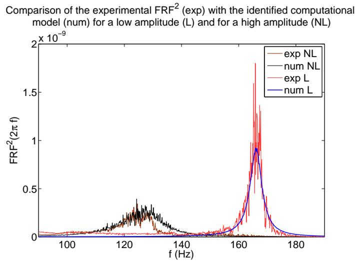
Figure 6: Comparison of the experimental  $FRF^2$  (exp) with the identified computational model (num) for a low amplitude (L) and for a high amplitude (NL).
