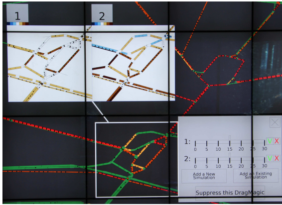
Figure 6. A DragMagic with two forecast visualizations (top left) linked to its area of focus (inside white rectangle), and its menu open (right).
