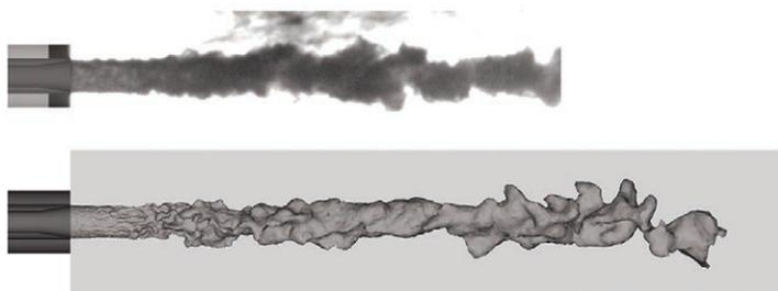
Figure 13 – Comparison between an experimental backlighting image of the A60 case [18] and a 200 kg/m<sup>3</sup> isodensity surface LES snapshot
