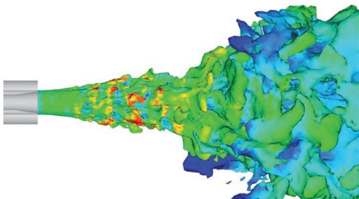
Figure 14 – 1500 K isotherm surface LES snapshot
