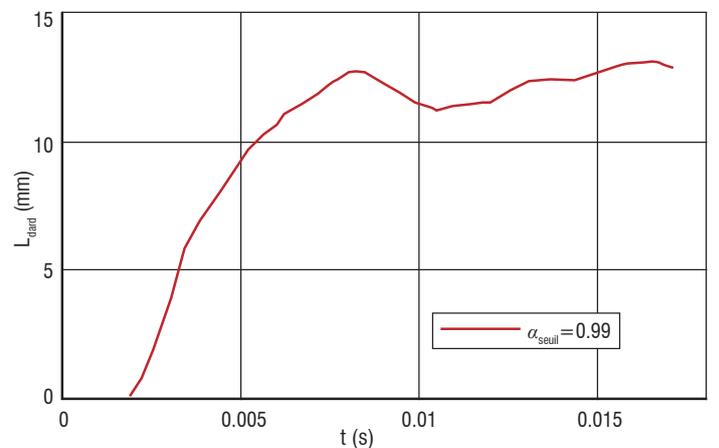
Figure 5 – Time evolution of pressure, temperature, volume fractions and penetration depth
