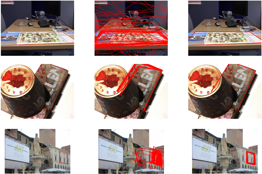
Figure 7: poster, book, pot, and tower datasets. From left to right: query camera and hand-picked scene edges; reprojection of these edges with 100 pose estimations without synthetic patches; reprojection of these edges with 100 pose estimations when using synthetic patches.
