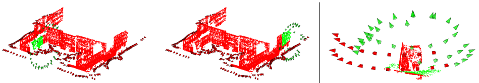
Figure 2: Virtual viewpoint positioning relative to some of the segmented patches (green points). In the left scene, only two rings of virtual viewpoints (in green) are added as the other potential viewpoints would have been close to existing viewpoints (in red).
