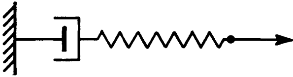
Fig. 2. Dashpot and spring in series, representing the operator (6.2) (Maxwell element).
