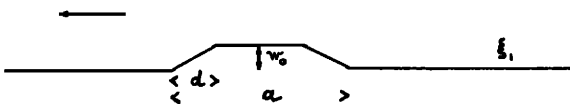
Fig. 1. Cross section along \xi_1 axis, showing velocity amplitude distribution over square membrane.
