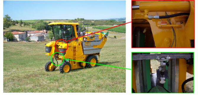
Fig. 6. Experimental vehicle equipped with low cost sensors used for observation: IMU (top right) and speed sensor (bottom right)
