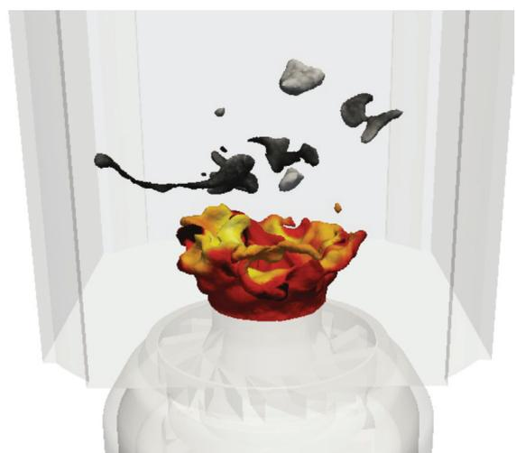
Figure 6 - LES of the DLR swirled turbulent flame [130]. Isocontour of temperature colored by the axial velocity (red-to-yellow) and soot ligaments colored by their number density (black-to-white).
