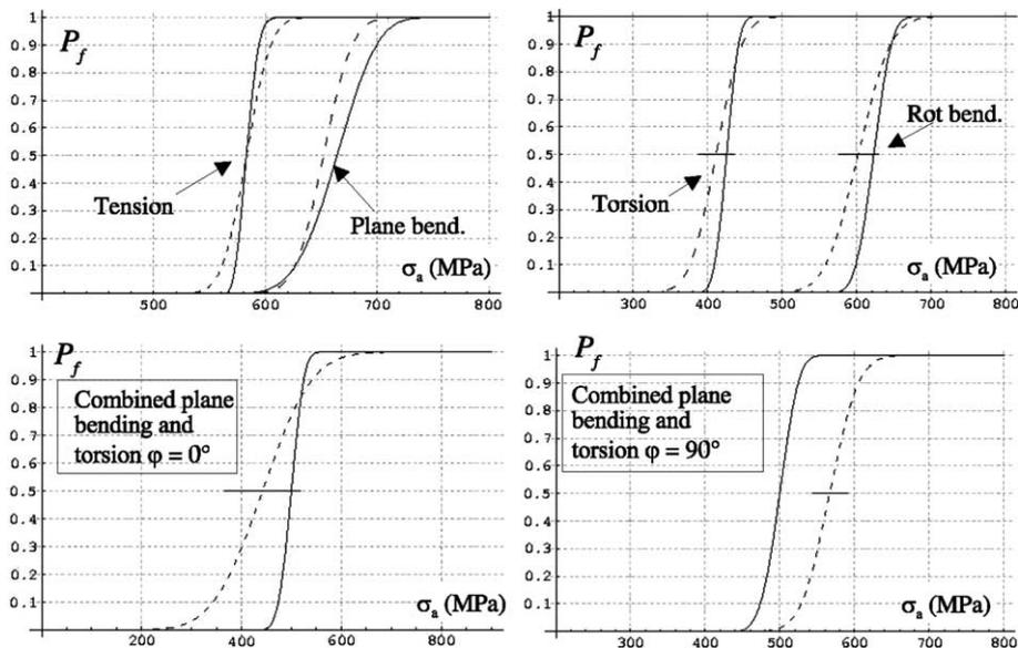
Fig. 2. Fatigue strength probability distributions  $P_f$  versus stress amplitude  $\sigma_a$  for smooth specimens in Ti-6Al-4V alloy. For combined plane bending and torsion:  $R_\sigma = -1$ ,  $\sigma_a/T_a = 1.732$  (full line: theoretical predictions, dashed line: experimental distributions).
