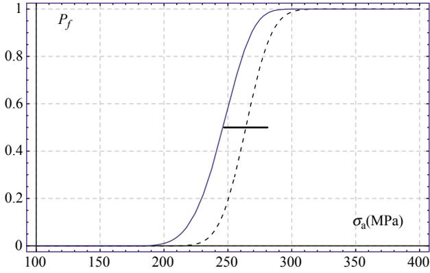
Fig. 4. Fatigue strength probability distributions  $P_f$  versus stress amplitude  $\sigma_a$  for smooth specimens in C20 steel loaded under fully reversed combined plane bending and torsion with a phase-shift of  $90^\circ$  and  $\sigma_a/\tau_a=1.78$  (full line: theoretical predictions, dashed line: experimental distributions).
