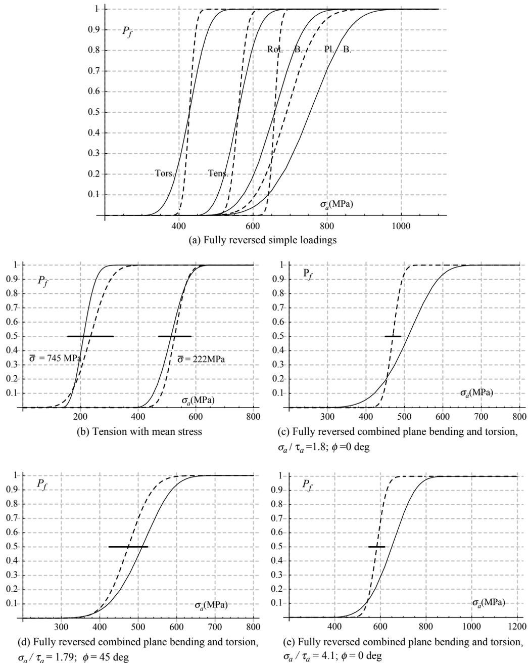
Fig. 3. Fatigue strength probability distributions  $P_f$  versus stress amplitude  $\sigma_a$  for smooth specimens in 30NiCrMo16 steel (full line: theoretical predictions, dashed line: experimental distributions).
