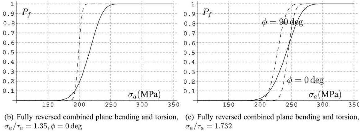
Fig. 6. Fatigue strength probability distributions  $P_f$  versus stress amplitude for smooth specimens in EN-GJS800-2 SG cast iron (full line: theoretical predictions, dashed line: experimental distributions).
