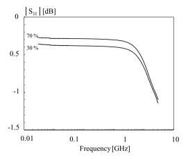
Fig. 4. Measured reflection coefficient  $\underline{S}_{II}$  for suspensions of microalgae with different lipid contents.
