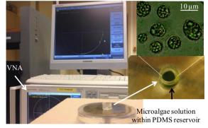
Fig. 1. Photography of the test bench. The inset is optical microscope photography of suspended microalgae solution.  $(1ml - number of cells \sim 7 \times 10^7).$
