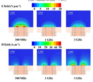
Figure 2: Magnitude of the electrical and magnetic field distributions at the test frequencies 0.3, 1 and 3 GHz in cross-section (on conductive medium; 0.1 S.m<sup>-1</sup>).
