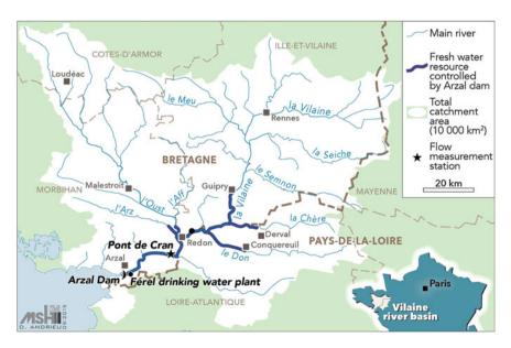
Fig. 6.2 Location of the Vilaine catchment, the Arzal dam and the zone of influence of the dam in the upper part of the riverbed
