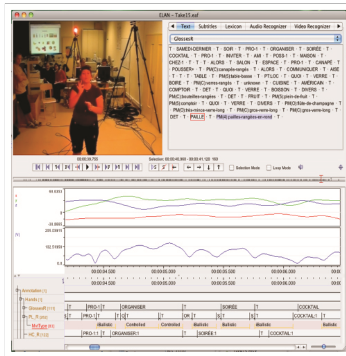
Fig. 4 Phonetic-based annotation [8]; ELAN can be configured to show motion captured data that is synchronized with the annotation timeline [6].
