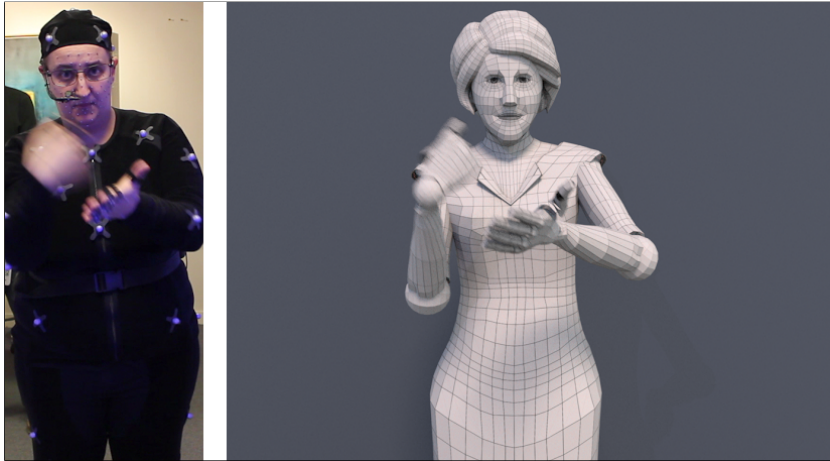
Fig. 3 Motion capture session: the real signer from the recorded video (left) and the 3D mesh of the corresponding virtual signer (right).
