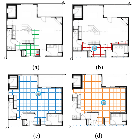
Fig. 10. ILP solution for Z_{c1,1} . (a) Zone covered by the sensor of type h = 1 . (b)–(d) Zone covered by the three sensors of type h = 4 .
