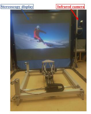
Fig. 2. Evr@ virtual reality platform with the 6 DoF mechanical system
