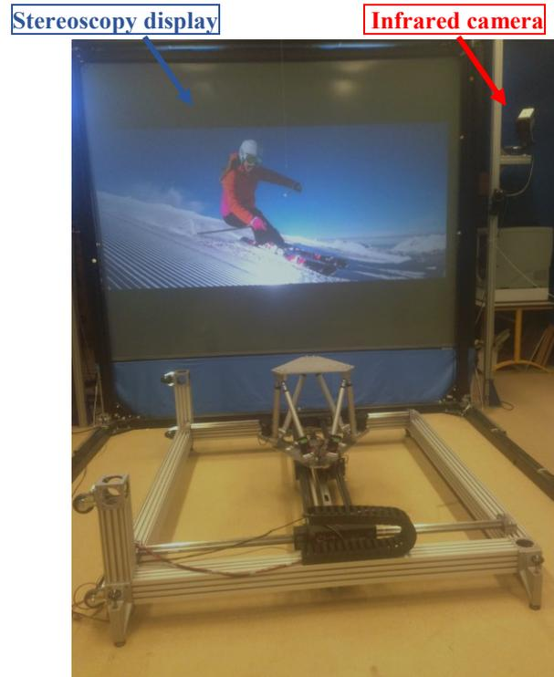
Fig. 2. Evr@ virtual reality platform with the 6 DoF mechanical system
