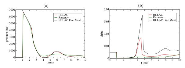
Figure 16: Cylindrical underwater explosion near a planar wall: comparison of the time evolutions of the pressure (a) and the gas volume fraction (b) obtained with the HLLAC and Rusanov schemes.
