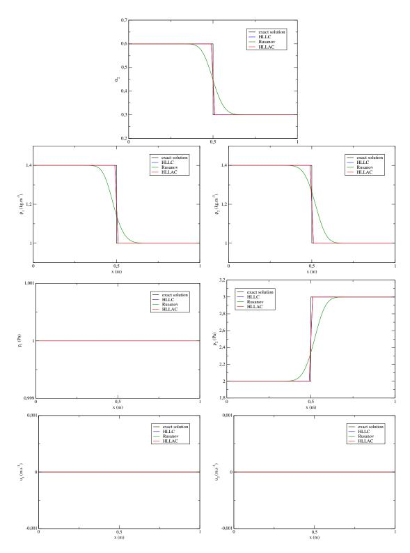
Figure 7: Comparison between analytical and numerical solutions on Test 3 with 100 cells at time  $t_f = 0.05s$ . From the top to the bottom right:  $\alpha_2, \rho_1, \rho_2, p_1, p_2, u_1, u_2$  vs x.
