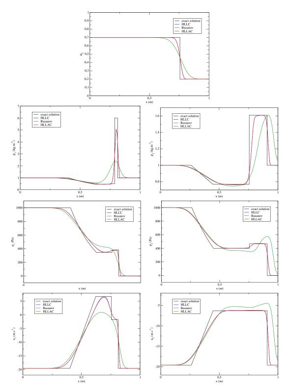
Figure 8: Comparison between analytical and numerical solutions on Test 4 with 100 cells at time  $t_f = 0.007s$ . From the top to the bottom right:  $\alpha_2, \rho_1, \rho_2, p_1, p_2, u_1, u_2$  vs x.
