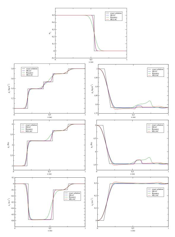
Figure 11: Comparison between analytical and numerical solutions on Test 6 with 200 cells at time  $t_f = 0.15s$ . From the top to the bottom right:  $\alpha_2, \rho_1, \rho_2, p_1, p_2, u_1, u_2$  vs x.
