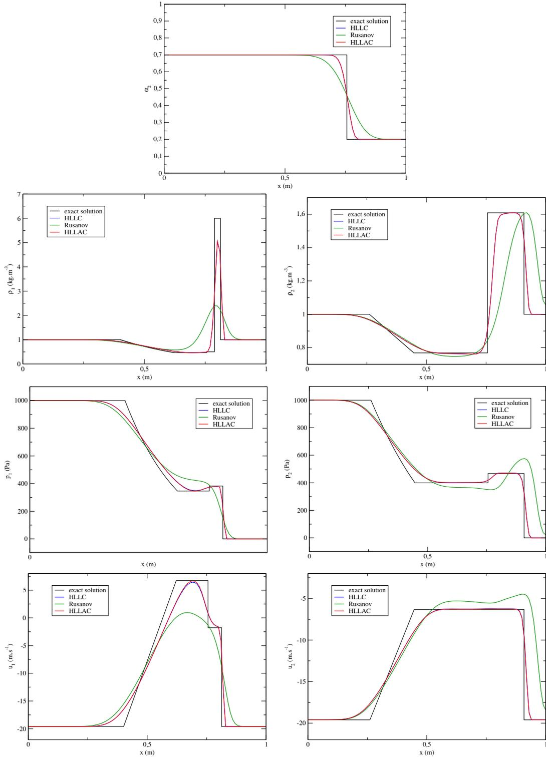
Figure 8: Comparison between analytical and numerical solutions on Test 4 with 100 cells at time  $t_f = 0.007s$ . From the top to the bottom right:  $\alpha_2, \rho_1, \rho_2, p_1, p_2, u_1, u_2$  vs  $x$ .
