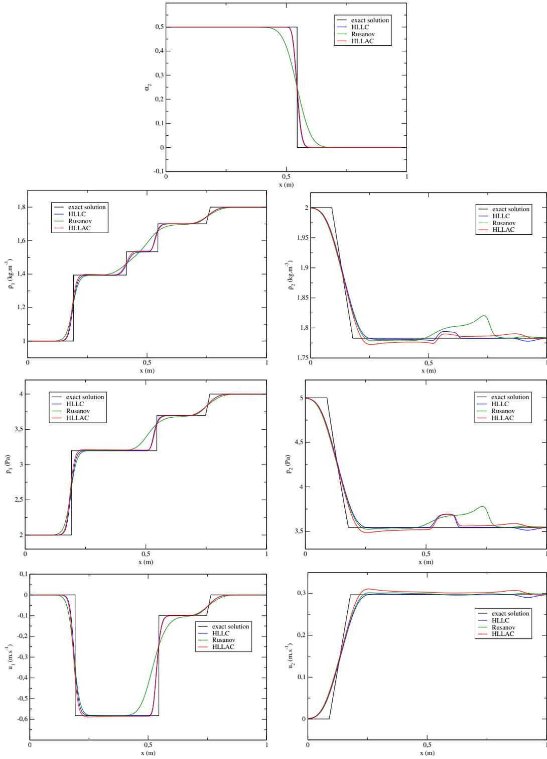
Figure 11: Comparison between analytical and numerical solutions on Test 6 with 200 cells at time  $t_f = 0.15s$ . From the top to the bottom right:  $\alpha_2, \rho_1, \rho_2, p_1, p_2, u_1, u_2$  vs  $x$ .
