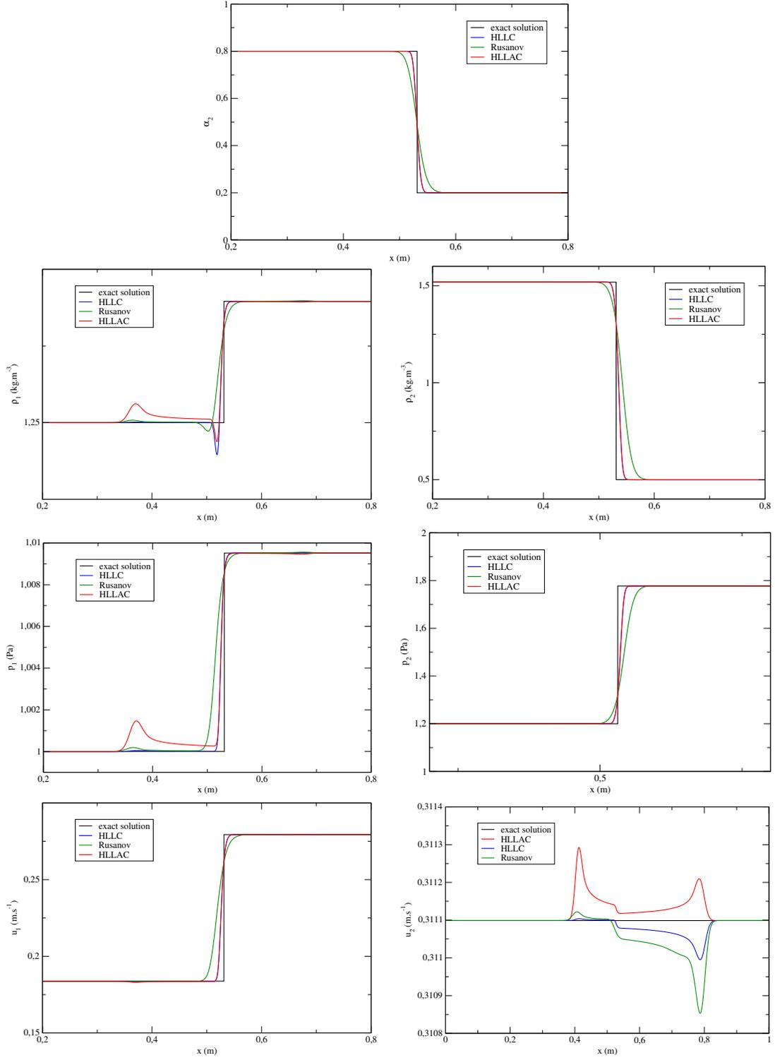
Figure 2: Comparison between analytical and numerical solutions on Test 1 with 1000 cells at time  $t_f = 0.1s$ . From the top to the bottom right:  $\alpha_2, \rho_1, \rho_2, p_1, p_2, u_1, u_2$  vs  $x$ .
