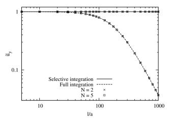
Fig. 7. Transverse displacement ratio  $\tilde{u}_y = u_y(l/2, 0, 0)/u_y^{\text{Nav}}(l/2, 0, 0)$  versus l/a via linear elements, N = 2 and 5. The figure is the same for the FEM as well as FEM PGD solution regardless the value of  $N_c$ .
