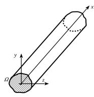
Fig. 1. Beam geometry and reference system.
