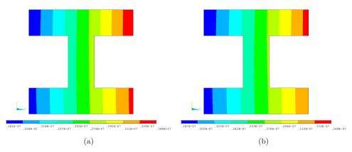
Fig. 14. Transverse displacement  $u_y$  [m] over the cross-section at x/l = 0.5 via (a) FEM 3D-R and (b) PGD FEM 1D (cubic elements, N = 17 and  $N_c = 7$ ) solutions. Simply supported beam with l/a = 10.
