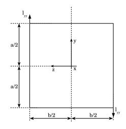
Fig. 10. Square cross-section geometry and line torsional loads.
