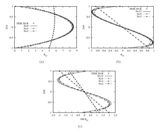
Fig. 9. Shear stresses variation over the cross-section: (a)  $\overline{\sigma}_{xy}(0, y, +b/2)$ , (b)  $\overline{\sigma}_{xz}(0, a/2, z)$  and (c)  $\overline{\sigma}_{yz}(l/2, 0, z)$ . Simply supported beam, l/a = 10, cubic elements and  $N_c = 7$ .
