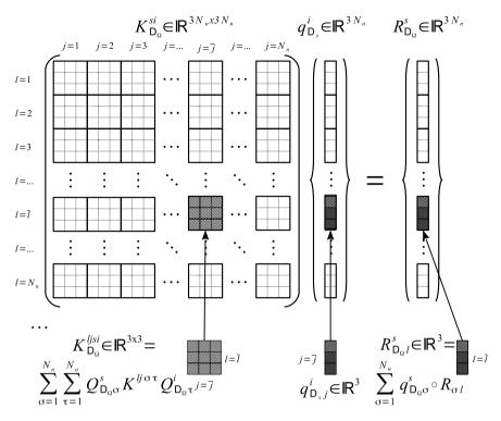
Fig. 3. Assembling procedure of the axial finite element problem  $\mathcal{D}_x$  at element level.
