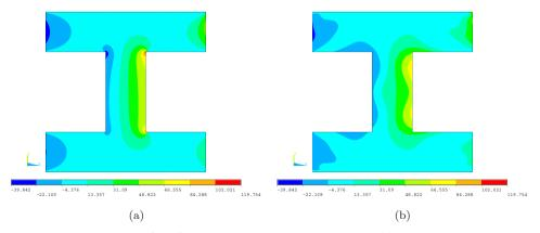
Fig. 19. Shear stress  $\sigma_{xy}$  [MPa] over the cross-section at x/l = 0 via (a) FEM 3D-R and (b) PGD FEM 1D (cubic elements, N = 17 and  $N_c = 7$ ) solutions. Simply supported beam with l/a = 10.
