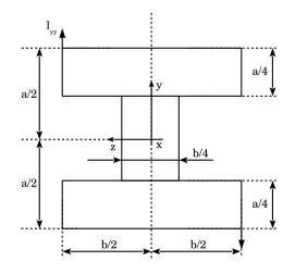
Fig. 11. I-shaped cross-section geometry and line load.
