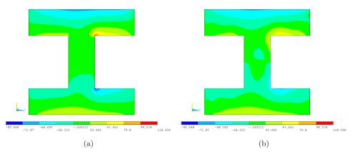
Fig. 20. Shear stress  $\sigma_{xz}$  [MPa] over the cross-section at x/l = 0 via (a) FEM 3D-R and (b) PGD FEM 1D (cubic elements, N = 17 and  $N_c = 7$ ) solutions. Simply supported beam with l/a = 10.
