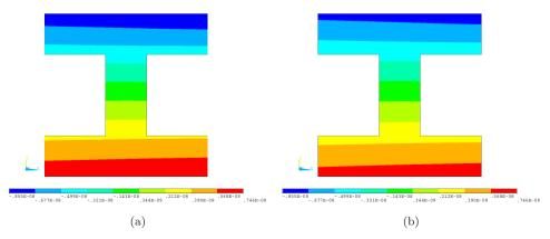
Fig. 13. Transverse displacement  $u_z$  [m] over the cross-section at x/l = 0.5 via (a) FEM 3D-R and (b) PGD FEM 1D (cubic elements, N = 17 and  $N_c = 7$ ) solutions. Simply supported beam with l/a = 10.
