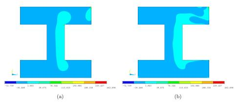
Fig. 16. Normal stress  $\sigma_{yy}$  [MPa] over the cross-section at x/l = 0.5 via (a) FEM 3D-R and (b) PGD FEM 1D (cubic elements, N = 17 and  $N_c = 7$ ) solutions. Simply supported beam with l/a = 10.
