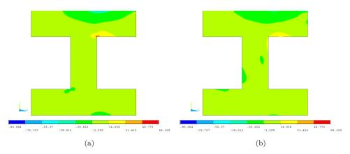
Fig. 17. Normal stress  $\sigma_{zz}$  [MPa] over the cross-section at x/l = 0.5 via (a) FEM 3D-R and (b) PGD FEM 1D (cubic elements, N = 17 and  $N_c = 7$ ) solutions. Simply supported beam with l/a = 10.
