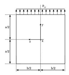
Fig. 4. Square cross-section geometry and surface bending load.
