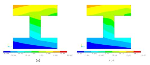
Fig. 15. Axial stress  $\sigma_{xx}$  [MPa] over the cross-section at x/l = 0.5 via (a) FEM 3D-R and (b) PGD FEM 1D (cubic elements, N = 17 and  $N_c = 7$ ) solutions. Simply supported beam with l/a = 10.
