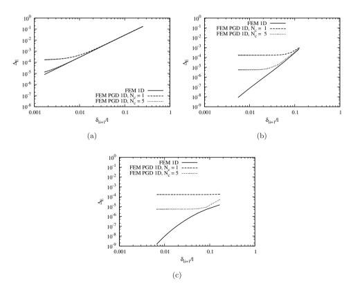
Fig. 5. Strain energy relative error  $\Delta_E$  versus the normalized distance  $\delta_{ii+1}/l$  between two consecutive nodes for (a) linear, (b) quadratic and (c) cubic element. Simply supported beam, l/a = 10 and N = 2.
