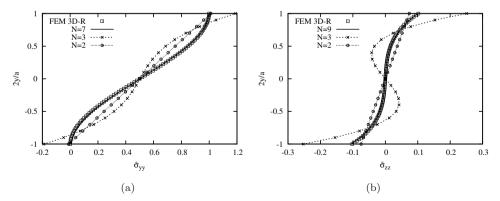
Fig. 8. Normal stresses variation over the cross-section: (a)  $\overline{\sigma}_{yy}(l/2, y, b/2)$  and (b)  $\overline{\sigma}_{zz}(l/2, y, 0)$ . Simply supported beam, l/a = 10, cubic elements and  $N_c = 7$ .
