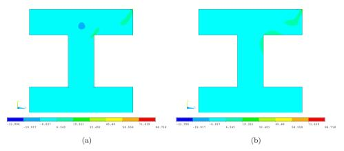
Fig. 18. Shear stress  $\sigma_{yz}$  [MPa] over the cross-section at x/l = 0.5 via (a) FEM 3D-R and (b) PGD FEM 1D (cubic elements, N = 17 and  $N_c = 7$ ) solutions. Simply supported beam with l/a = 10.
