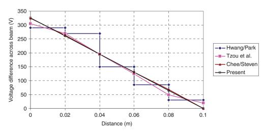
Figure 14. Voltage difference across the thickness of PVDF at various points along the length of the beam — PVDF bimorph beam — sensor configuration.
