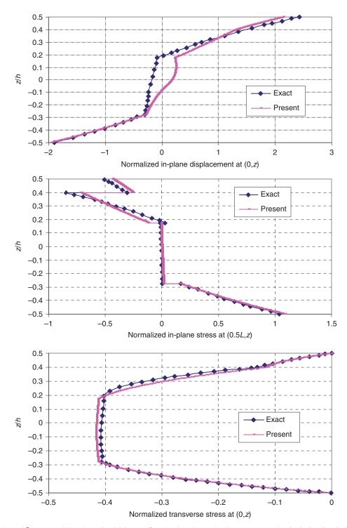
**Figure 5.** Distribution of  $\bar{u}_1$ ,  $\bar{\sigma}_{11}$ , and  $\bar{\tau}_{13}$  along the thickness (S=4) – four-layered substrate composite [pz/0°/90°/90°/0°].
