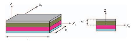
Figure 1. The laminated piezoelectric beam and coordinate system.
