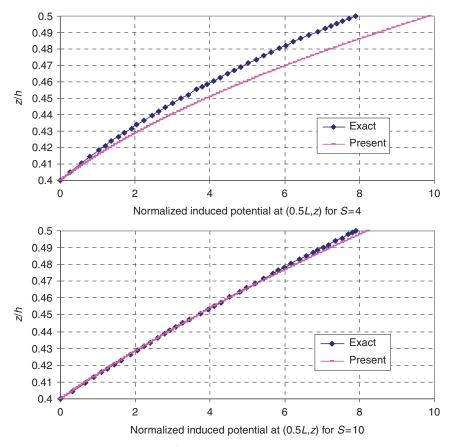
**Figure 7.** Distribution of the normalized sensory potential  $(\bar{\phi})$  along the sensor layer – four-layered substrate composite  $[pz/0^{\circ}/90^{\circ}/90^{\circ}/90^{\circ}]$ .
