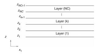
Figure 2. Coordinate system of the laminated piezoelectric beam.
