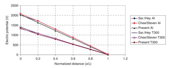
Figure 12. Voltage difference across the piezoelectric material as a function of normalized length of the cantilever beam — sensor configuration.
