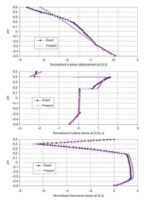
**Figure 8.** Distribution of  $\tilde{u}_1$ ,  $\tilde{\sigma}_{11}$ , and  $\tilde{\tau}_{13}$  along the thickness (S = 4) – four-layered substrate composite [pz/0°/90°/90°/0°].
