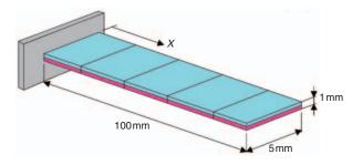
Figure 13. Cantilever piezoelectric bimorph beam.
