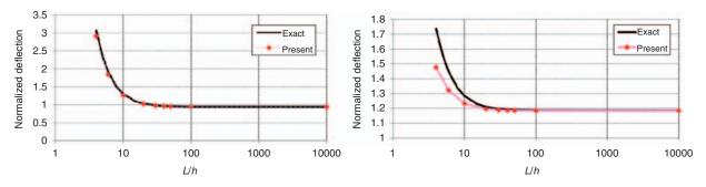
**Figure 4.** Distribution of the non-dimensional maximum displacement  $\tilde{u}_3(0.5L, 0)$  with respect to aspect ration L/h – four-layered substrate composite  $\lceil pz/0^{\circ}/90^{\circ}/90^{\circ}/90^{\circ} \rceil$  left (sensory beam) – right (actuated beam).
