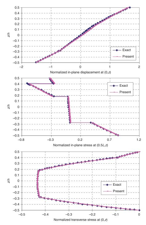
**Figure 6.** Distribution of  $\bar{u}_1$ ,  $\bar{\sigma}_{11}$ , and  $\bar{\tau}_{13}$  along the thickness (S = 10) – four-layered substrate composite [pz/0°/90°/90°/0°].
