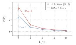
(b) Global buckling vs aspect ratio
