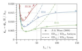
**Fig. 6.** Fagerberg case study: critical strain vs buckling wavelength for three different core qualities.
