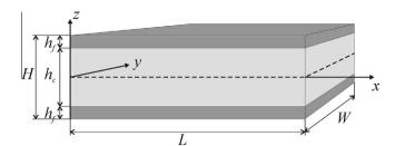
Fig. 1. Geometry of the symmetric sandwich plate
