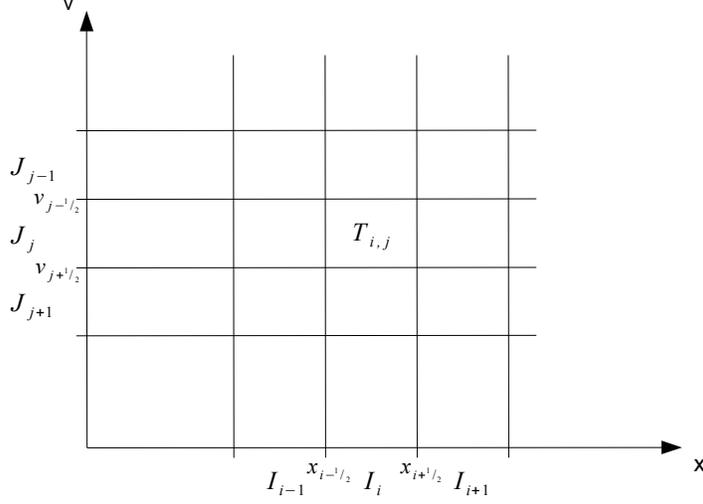
Figure 1: Mesh representation and notation.
