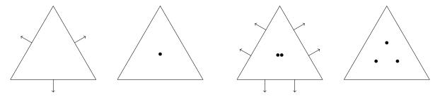
Figure 1: The mixed Raviart-Thomas finite element for l = 0 (left) and l = 1 (right)
