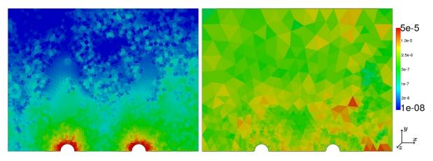
Figure 10: Spatial discretization error estimators at  $t_F$  on a fixed mesh (left, 29,275 dofs) and on the last mesh of an adaptive algorithm (right, 15,064 dofs)
