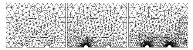
Figure 9: Initial mesh (left) and meshes at the end of the first (center) and the second (right) excavation in the adaptive algorithm
