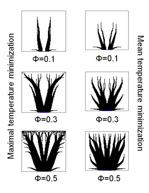
Figure 4: Optimal configuration proposed by GA for peak (left) or mean (right) temperature minimization  $(k_p/k_0=10; \phi \text{ from } 0.1 \text{ to } 0.5).$
