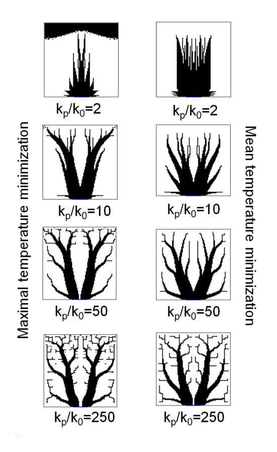
Figure 3: Optimal configuration proposed by GA for peak (left) or mean (right) temperature minimization  $(\phi=0.3; k_p/k_0 \text{ from } 2 \text{ to } 250).$
