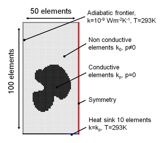
Figure 1: geometry and mesh used for this study. Note the symmetry on the right border.
