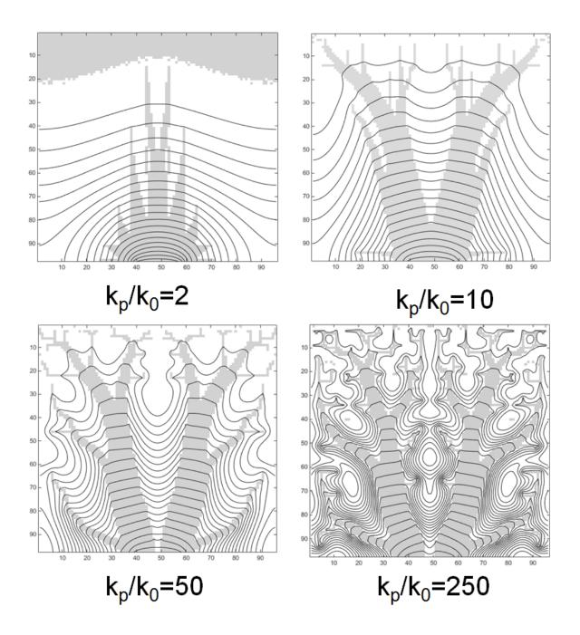
Figure 5: temperature isolines into the geometry converged for maximal (peak) temperature minimization with  $\phi = 0.3$  and  $k_p/k_0$  from 2 to 250.
