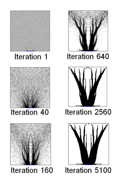
Figure 2: example of topology convergence for  $\phi = 0.3$  and  $k_p/k_0 = 10$  vs. generation (iteration). The conductive matter is black, the non conductive matter white. Grey levels indicate the cohabitation of several types of elements at a given position in the population for a given iteration.
